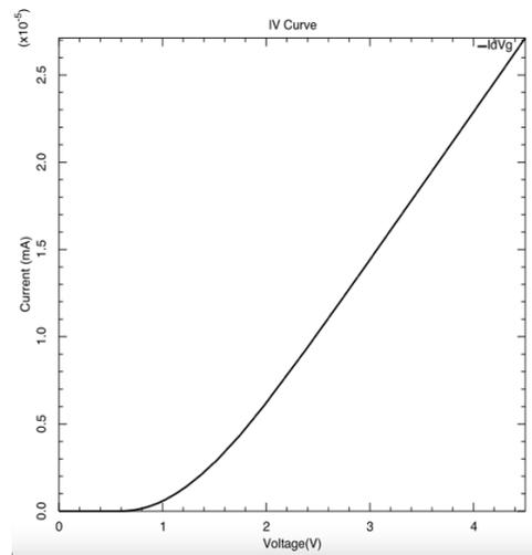
**EXAMPLE 3: GateCap.tcl, graphing Drain Current vs. Gate Voltage**
